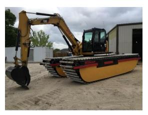
The Conservation Districts in Eastern Montana have a dredge that can work on a few sites but does not have the ability to work on over the 180 pump sites in a timely manner. The floating track hoe is expensive with an estimated cost \$400,000. A minimum of two would be required to clean pump sites in a timely manner. In addition, operating expenses to hire the track hoe to repair sites would be required. There are qualified contractors that could be hired to operate the equipment in the region.
