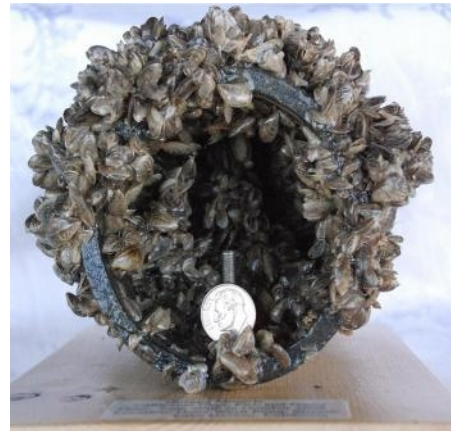
Zebra mussels have attached to this fatmucket mussel, a native mussel to Montana. (left) Photo by Rachael Ruggles at a MN lake. Clogging of pipe by mussels. Photo from Mussel Prevention Program, San Luis Obispo Co., Calif. (right)
